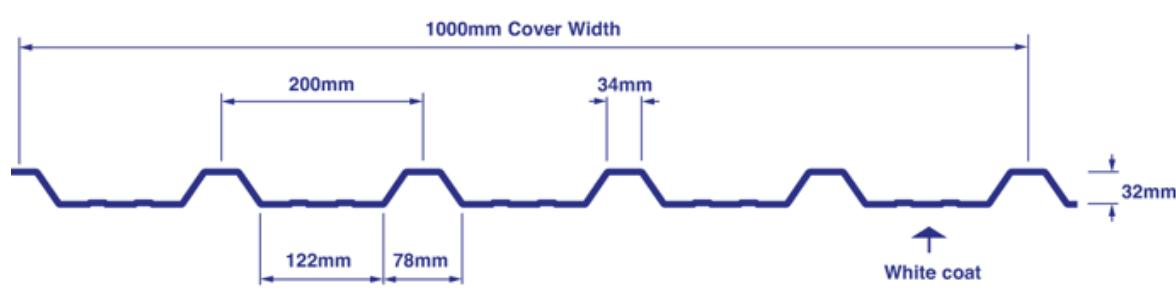
The Span Tables below have been created in accordance with EN 1993-1-3 (Eurocode EC3) and calculated by the Steel Construction Institute (SCI). The values are based on a maximum permitted deflection of Span/200 under imposed load.
