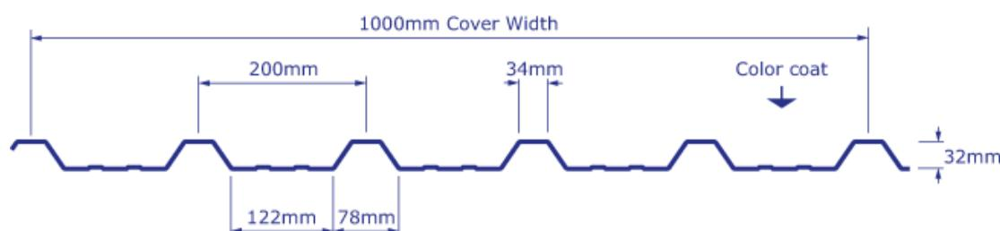
The Span Tables below have been created in accordance with EN 1993-1-3 (Eurocode EC3) and calculated by the Steel Construction Institute (SCI). The values are based on a maximum permitted deflection of Span/200 under imposed load.
